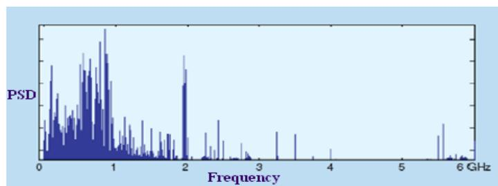
Fig. 1: Spectrum Utilization Measurement from 0-6 GHz [12]
