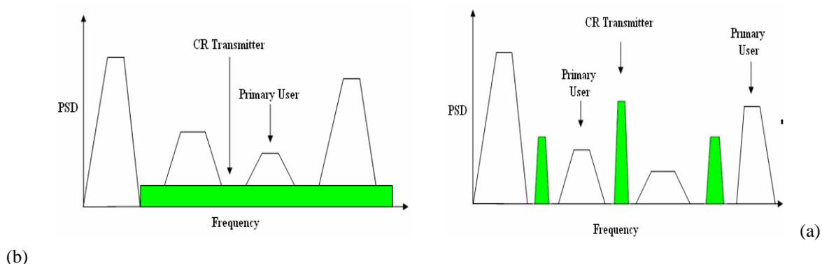
Fig.3 Spectrum Sharing approaches (a) Underlay (b) Overlay
