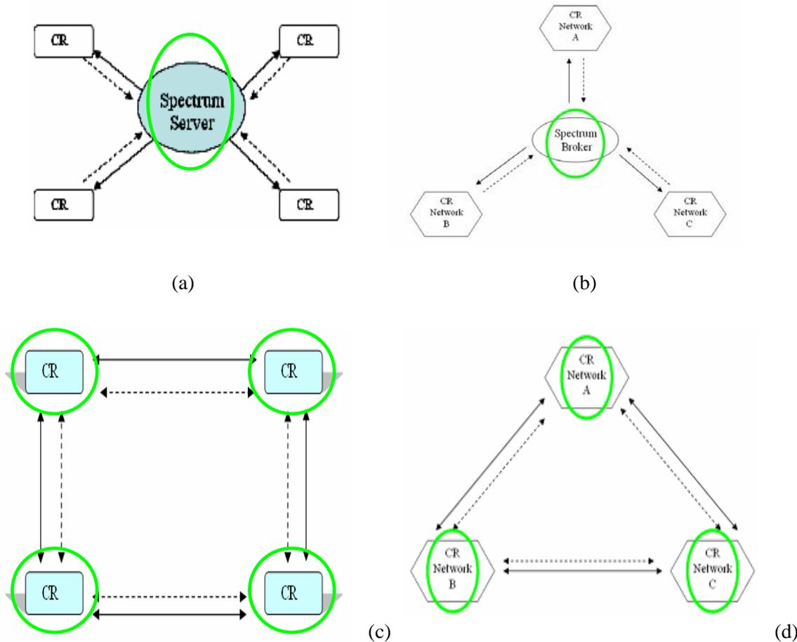
Fig. 4: Spectrum Sharing: Centralized Intra-network (a) Centralized Inter-network (b) Distributed Intra-network (c) Distributed Inter-network (d) [19]
