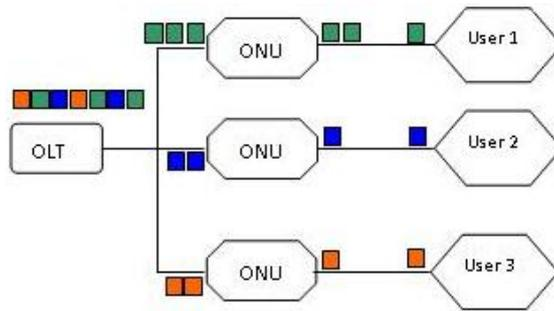
Fig. 1: downstream transmission
