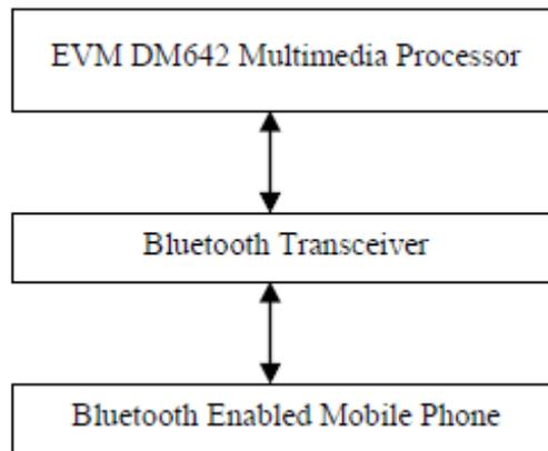
Fig. 2: Bluetooth Connection of Mobile phone with DM642
