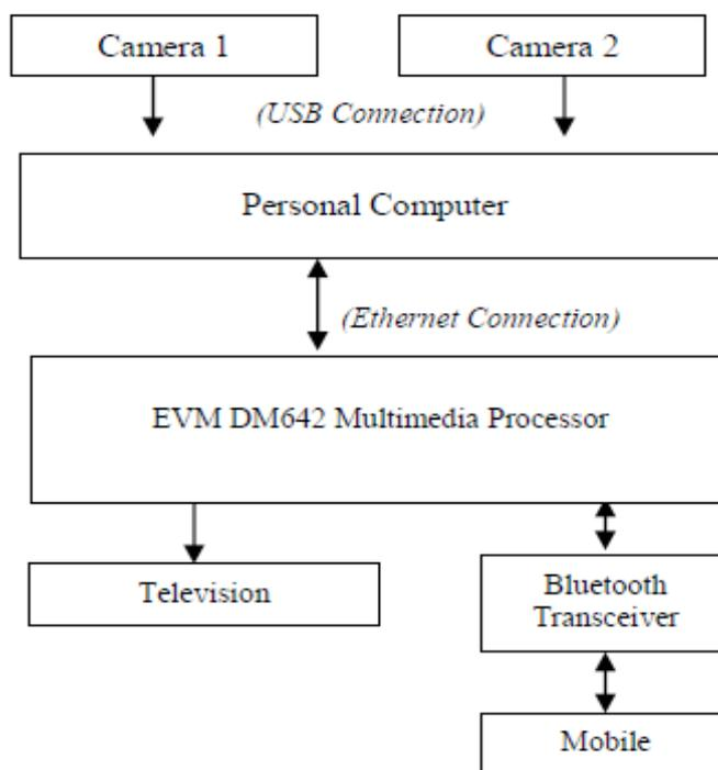
Fig. 1: Overall System Model
