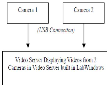
Fig. 3: Connection of cameras with the Video Server
