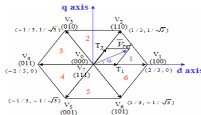
Fig. 7: Basic switching vectors and sectors
