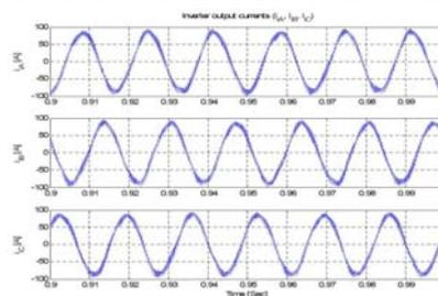
Fig. 8: Simulation results of inverter output currents
