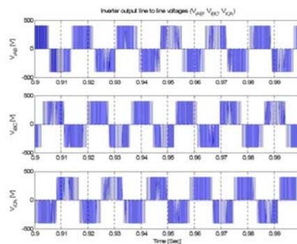
Fig. 7: Simulation results of inverter output line to line voltages
