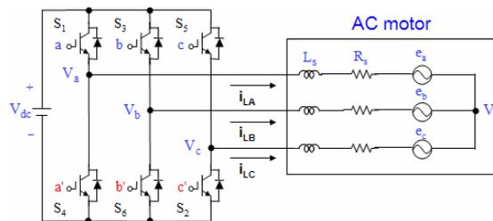
Fig 3. Three-phase voltage source PWM Inverter
