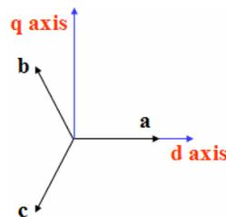
Fig. 6: The relationship of abc reference frame and stationary dq reference frame.
