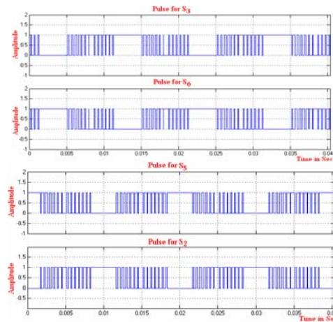
Fig. 9: Triggering SVPWM pulses for the VSI circuit from FPGA
