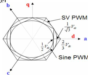
Fig. 5: Locus comparison of maximum linear control voltage in Sine PWM and SVPWM.
