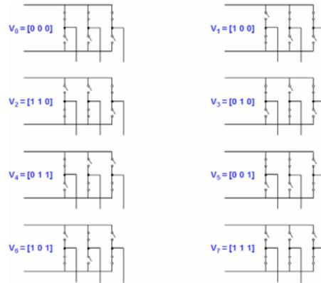
Fig. 4: The eight inverter voltage vectors ( $V_0$  to  $V_7$ )
