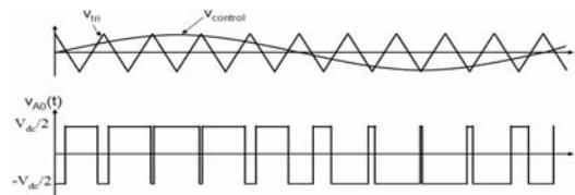
Fig 2. Pulse width modulation.
