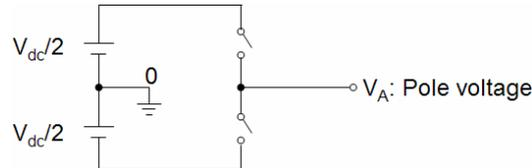
Fig 1. Circuit model of a single-phase inverter
