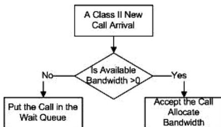
Fig. 1: Flow diagram of CAC
