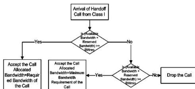
Fig. 2: Flow diagram for variable bandwidth processing of handoff call
