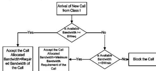
Fig.1: Flow diagram for variable bandwidth processing of new call
