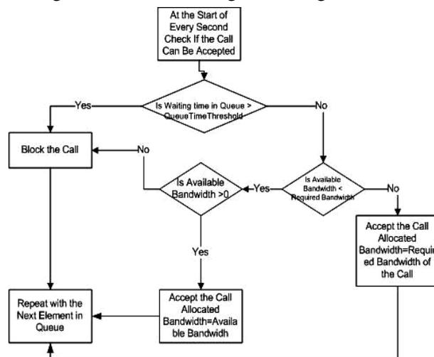
Fig. 2: Flow diagram of Queue processing in the cell
