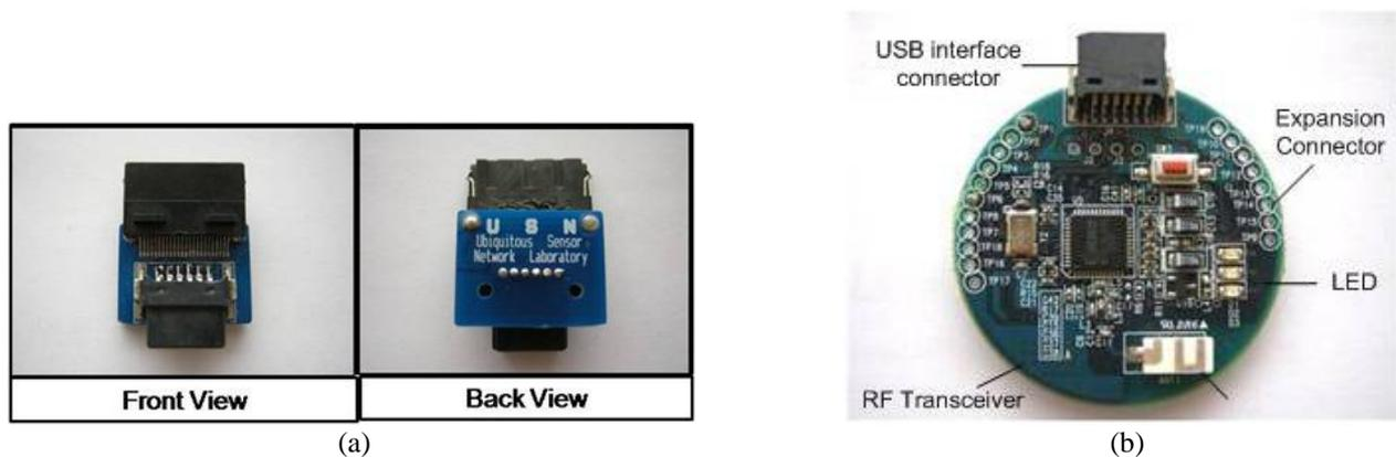
Fig. 4: Screen captured of our lab designed (a) RS-232 interface and (b) base station.
