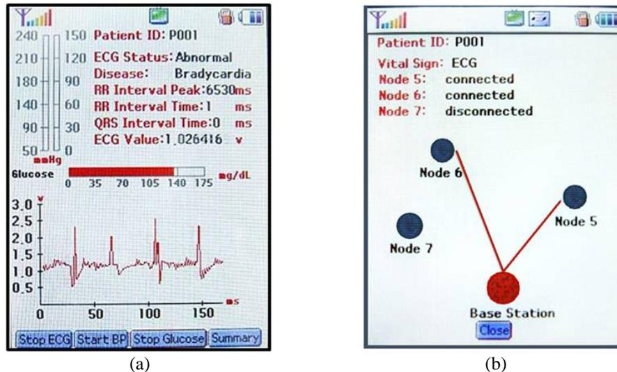
Fig. 7: (a) GUI displays ECG signals in waveform and blood glucose measure data in bar chart. (b) Network topology view of base station connects to sensor nodes are displayed.
