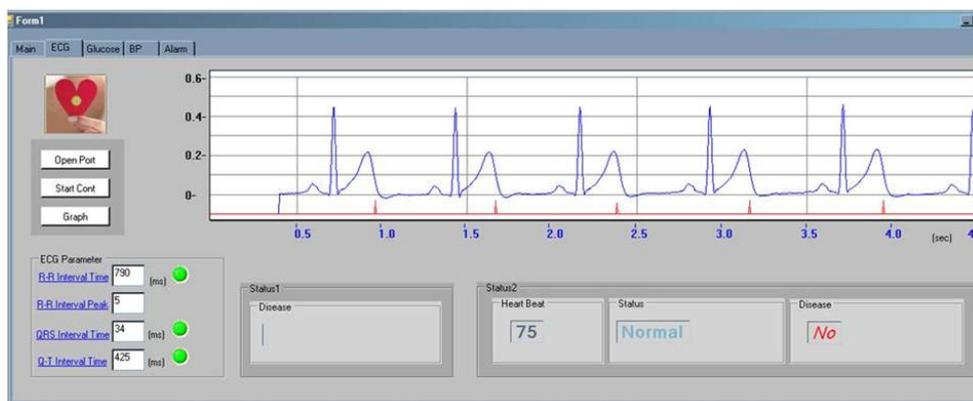
Fig. 5: Monitoring program analyzes ECG signals in desktop PC.
