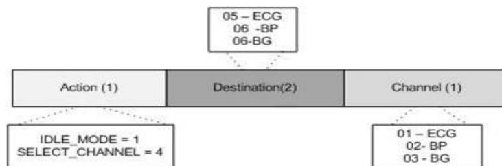
Fig. 2: Packet structure for command message.
