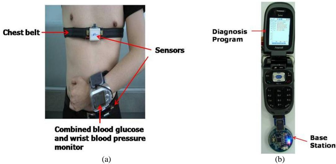
Fig. 6: (a) Tester wore medical monitor devices connect to sensors to measure vital signs health data. (b) Data are transmitted from sensors to cell phone through base station.
