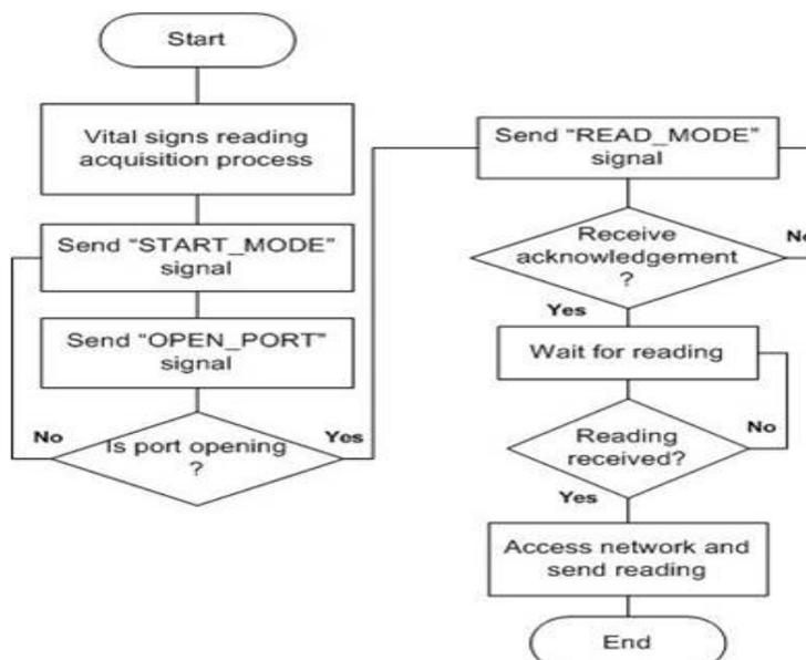
Fig. 3: Communication between medical monitor device and sensors flow chart.
