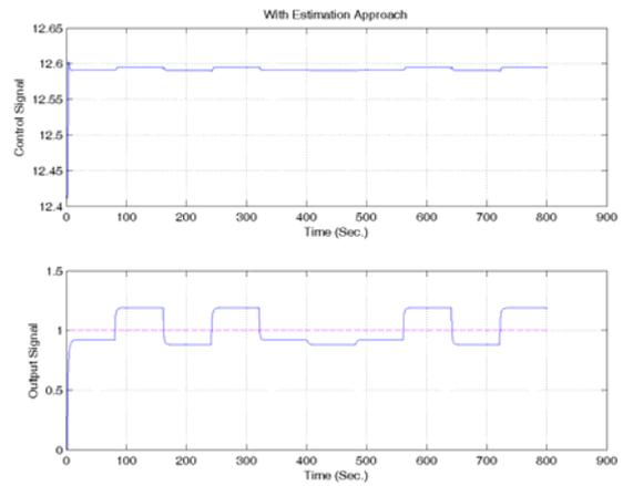
Figure 6 a) Engine speed and Throttle angle variations estimator method response
