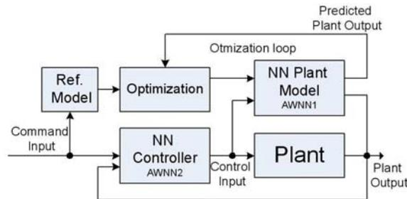
Figure2: A block diagram of the controller scheme
