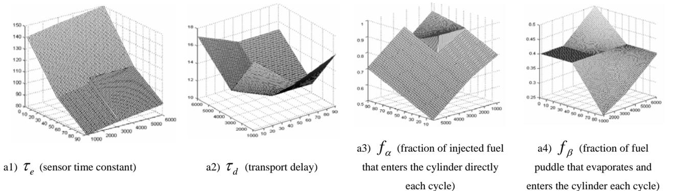
Figure 4 main parameters variations in work point space
