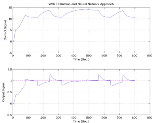
Figure 6 b) Engine speed and Throttle angle variations Neural Network method response
