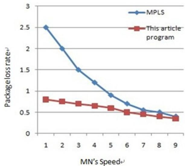
Fig. 7 Switching packet loss rate
