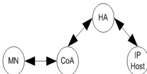
Fig. 1 the Communication Process of the Roaming MN Communicating With the IP Host
