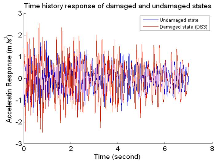
Fig. 4: Acceleration response at typical measurement point for damaged and undamaged state.
