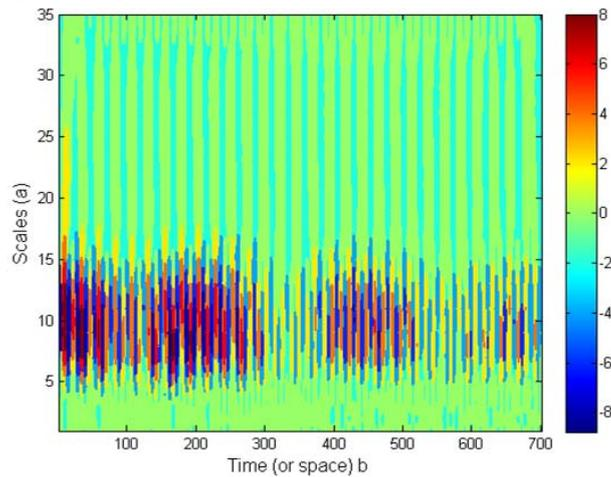
Fig. 5: Contour of difference between wavelet coefficient of damaged and undamaged state.
