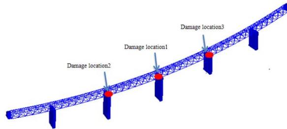
Fig. 2: Damage locations.
