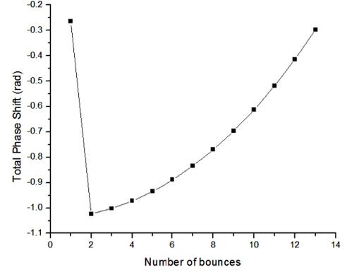
Fig. 3. Variation of net phase shift encountered by the interacting waves at each TIR bounce inside the tapered slab corresponding to the centre wavelength (7.521  $\mu\text{m}$ ) of the fundamental beam.
