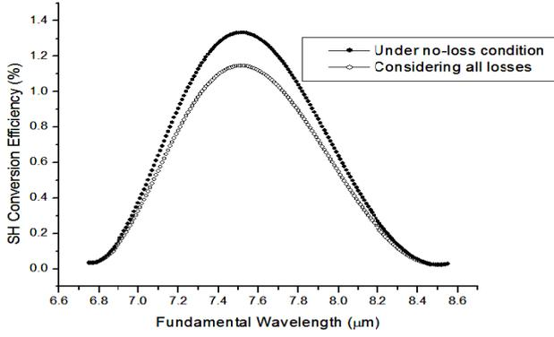
Fig. 2. Plot of SH efficiency vs input wavelength for the tapered ZnTe slab for  $\psi = 0.6$  rad,  $\phi_i = 1.1$  rad,  $L = 10$  mm,  $t_1 = 1000$   $\mu\text{m}$ , and  $t_2 = 1010$   $\mu\text{m}$ : (a) under no-loss condition and (b) considering all the losses (scattering, absorption, GH shift) encountered by the interacting waves.
