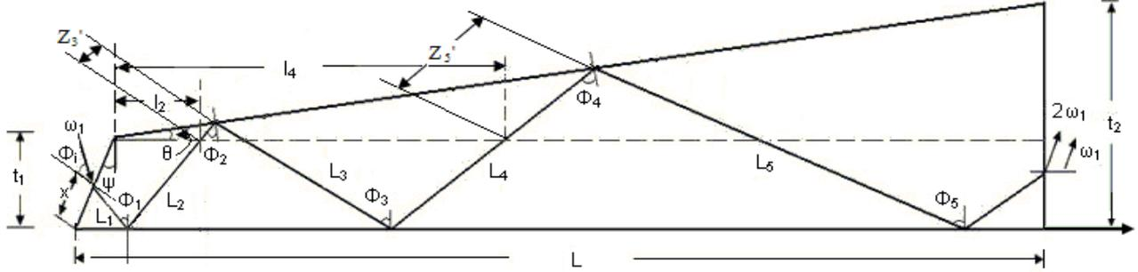
Fig. 1. Geometry of tapered semiconductor slab showing the scheme of second harmonic frequency conversion.
