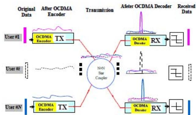
Fig. 1: Working principle of an OCDMA network .
