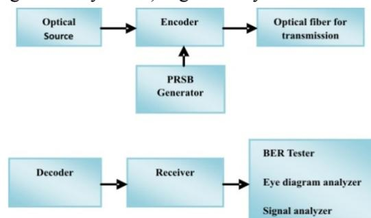
Fig. 2: Schematic Block Diagram for Spectral Phase Encoding Optical CDMA
