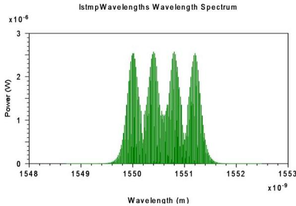
Fig. 4: Wavelength Spectrum for Spectral Phase Encoding Optical CDMA for Eight Users
