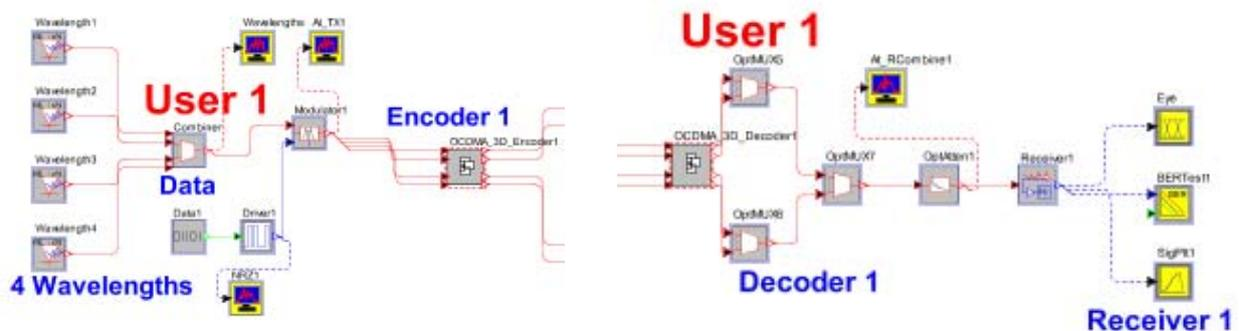
Fig.3: Simulation setup for Spectral Phase Encoding Optical CDMA system using for 1 User
