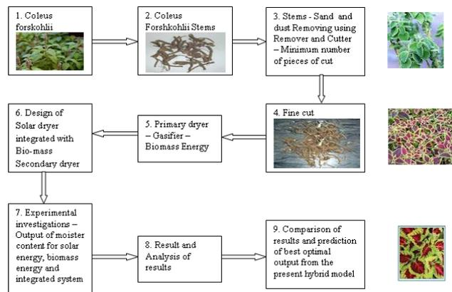
Fig.3. Work sequence of proposed Hybrid system
