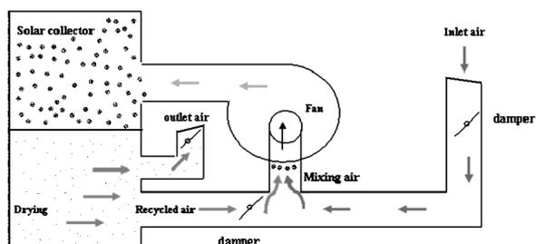
Fig.6. Model Design of Hybrid Solar -Biomass system
