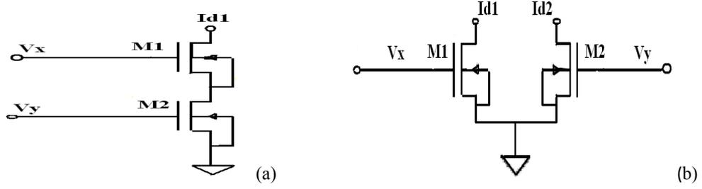
Fig.4: Shows the basic circuit configurations (a) Cascade structure (b) Parallel structure
