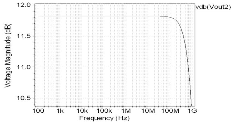
Fig.8 Frequency Response of Modified Multiplier
