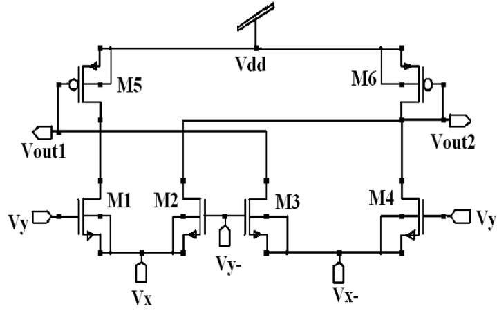
Fig.5: Modified Four Quadrant Multiplier Structure
