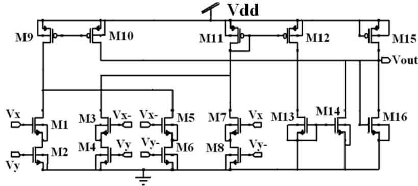
Fig.3: Schematic of Four Quadrant Voltage Mode Multiplier
