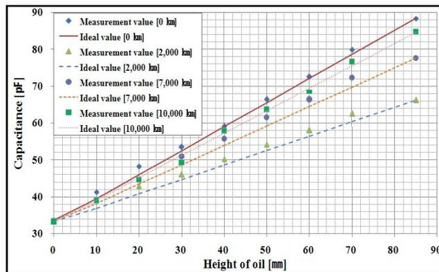
Fig. 7: Change of capacitance due to oil level and mileage
