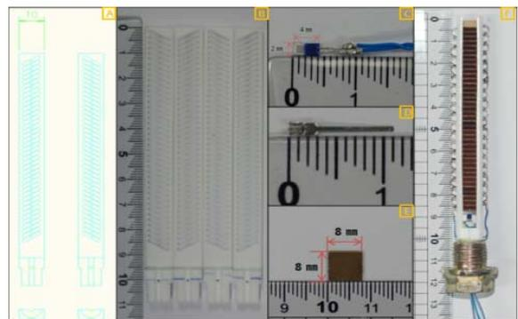
Fig. 3: Fabrication of engine oil degradation and level sensor (A: structural design, B: production structures, C: temperature sensor, D: electrode frame, E: electrode, F: sensor packaging).
