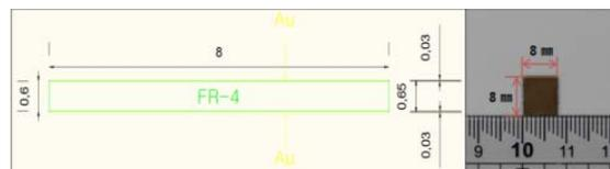
Fig. 1: Sensor electrode design.
