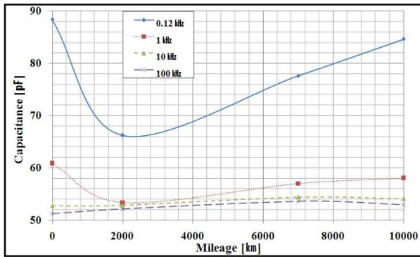
Fig. 5: change in capacitance due to frequency and mileage
