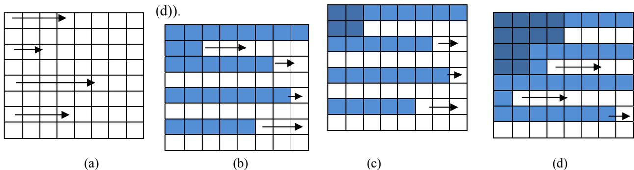
Fig. 3: Concurrent transformation a) Threads for each pair of row, b) Row transformation in progress, c) Column transformation done when pair of column elements are ready, d) Row and column transformation are in progress,
