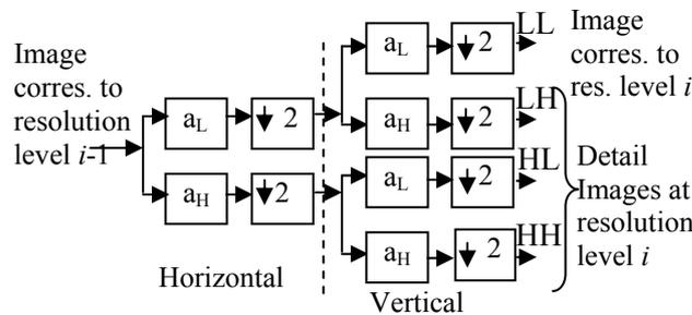
Figure 1. One Filter Stage in 2D Discrete Wavelet Transform
