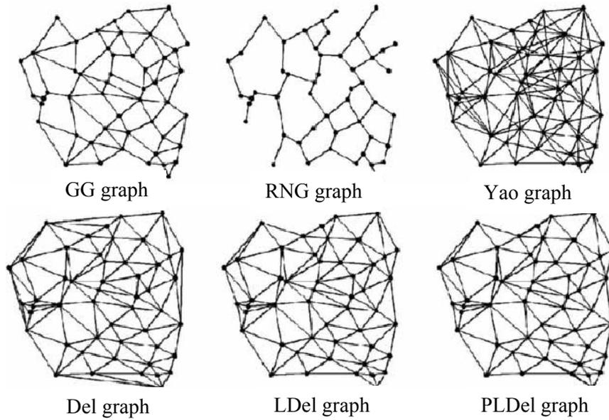
Fig.1. various planar network topologies
