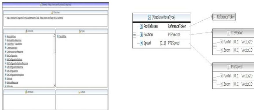
Fig. 1: An AbsoluteMove part of ONVIF XML schema
