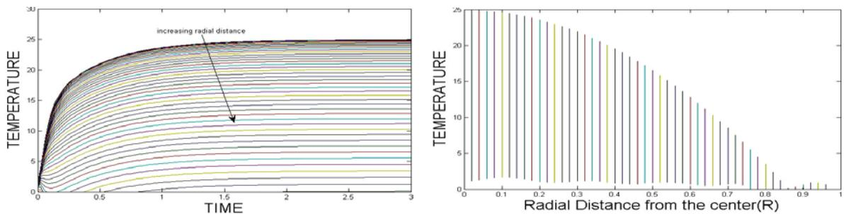
Fig 2 : AWG #1 Copper cable (variation of temperature with time) and (variation of temperature with radial distance)
