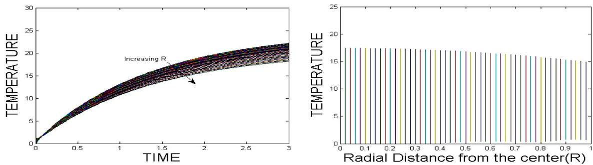
Fig 5 : AWG #1 Aluminium cable (variation of temperature with time) and (variation of temperature with radial distance)
