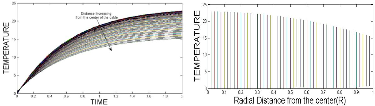
Fig 1 : AWG #6 Copper cable (variation of temperature with time) and (variation of temperature with radial distance)
