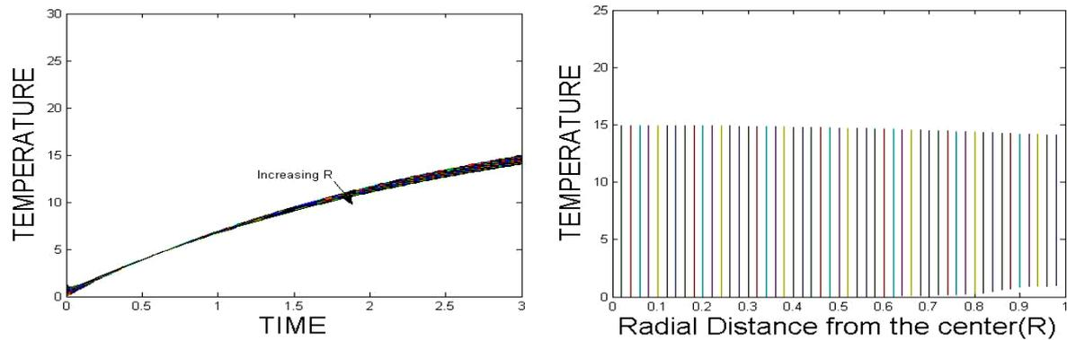
Fig 6 : AWG #10 Aluminium cable (variation of temperature with time) and (variation of temperature with radial distance)
