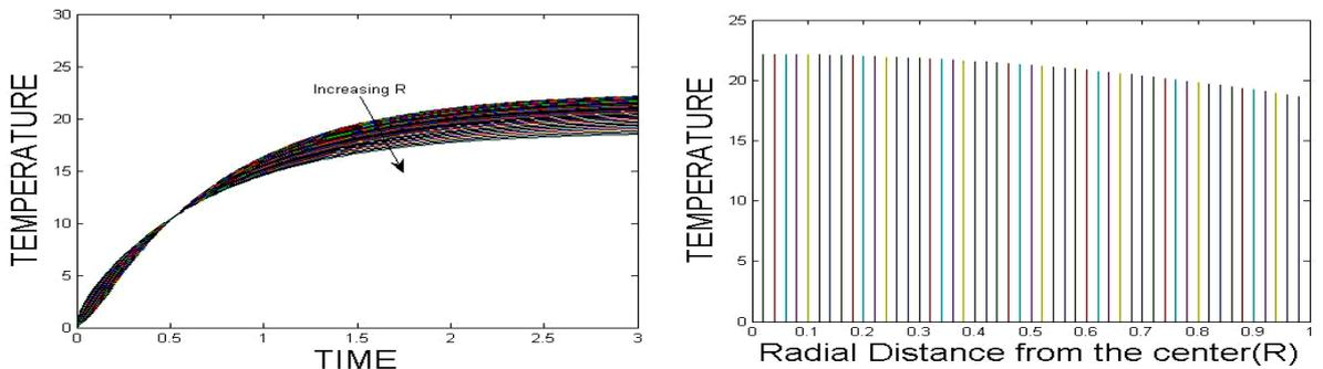
Fig 3 : AWG #10 Copper cable (variation of temperature with time) and (variation of temperature with radial distance)
