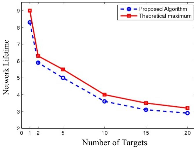
Figure 4: Effect of the number of targets on the network lifetime.
