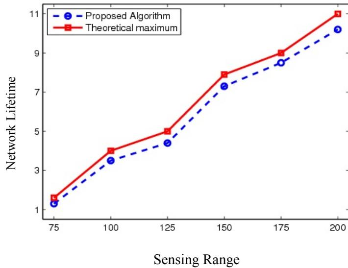
Figure 5: Effect of sensing ranges on the network lifetime.
