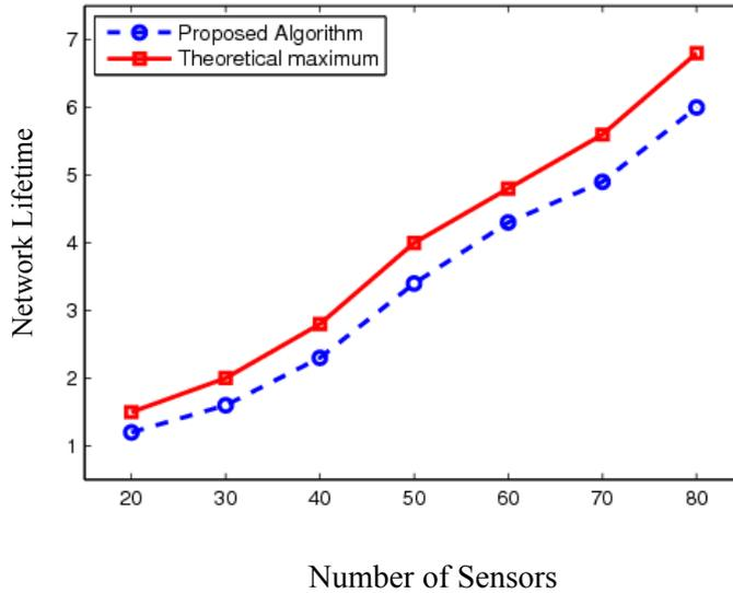
Figure 3: Effect of the number of sensors on the network lifetime.
