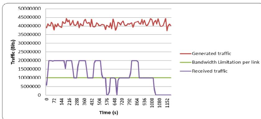
Fig. 9: Behaviour of EIGRP routing protocol under bandwidth limitation
