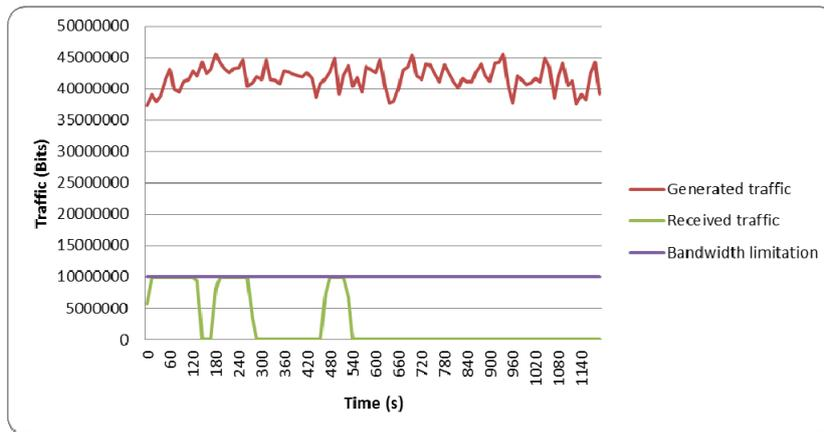
Fig. 5: EIGRP protocol behaviour under bandwidth limitation
