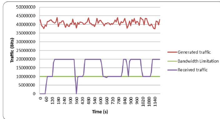
Fig. 8: Behaviour of OSPF routing protocol under bandwidth limitation
