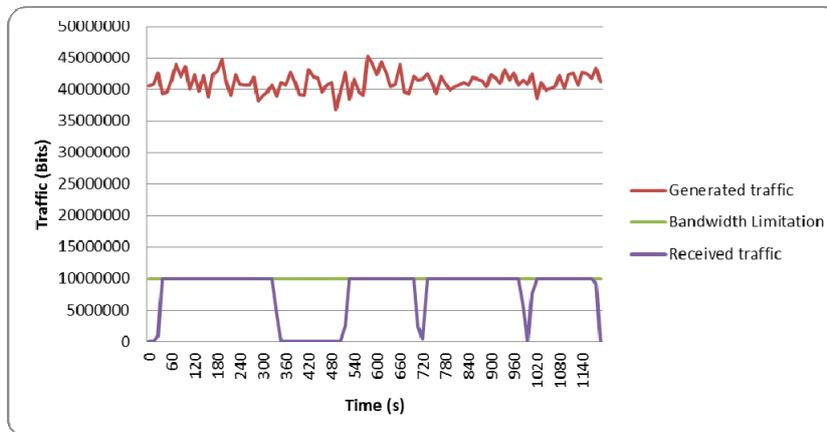
Fig. 6: OSPF protocol behaviour under bandwidth limitation
