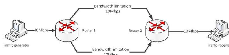
Fig. 7: Test platform for routing protocol behaviour – two links between routers
