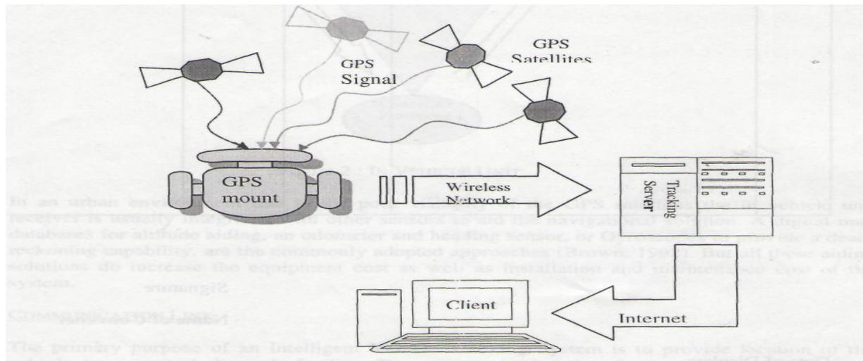
Figure 1: Standard IVTS Architecture
