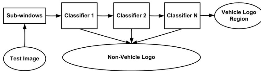
Fig. 3: Vehicle logo detection with cascade classifier
