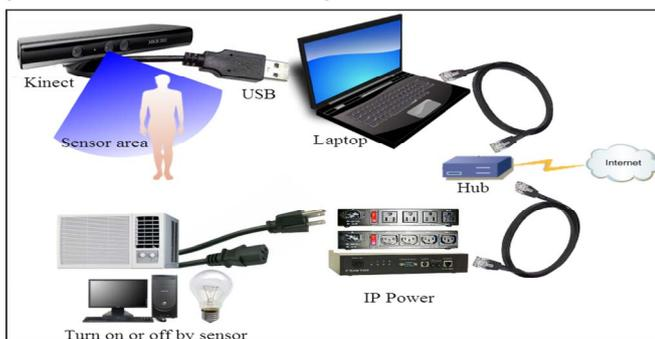
Fig.1 Structure of design: Using Kinect-IP Power System for Lab accessibility and energy saving improvement
