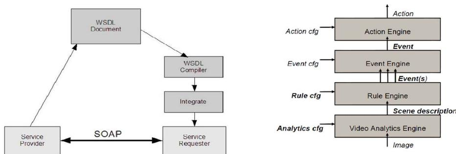
Fig.1. Standard web service configuration in ONVIF [3]
