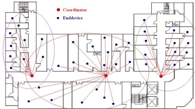
Fig. 4: Installation of sensor nodes in the 2nd floor of Electrical Engineering and Information Building.
