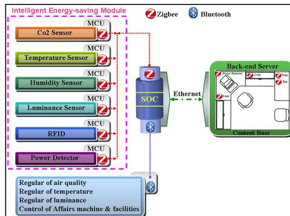
Fig. 2: System structure of intelligent energy conservation system.
