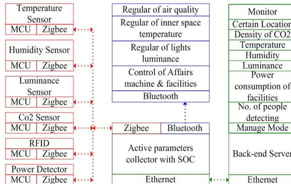
Fig. 1: Design concept of intelligent energy conservation system.
