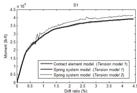
Fig.5 Comparison between the contact element model and spring system model
