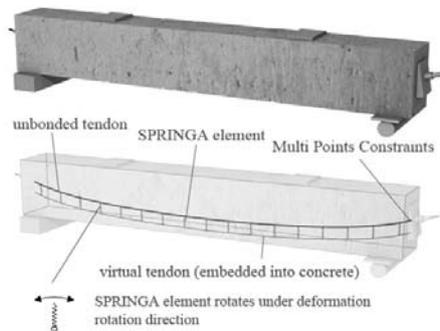
Fig.2 Modeling of unbonded PT tendons using the spring system model
