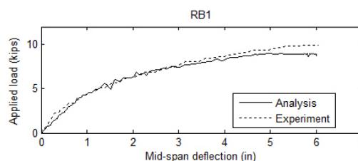
Fig.9 Modeling of unbonded PT tendons using the spring system model
