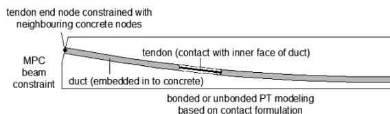
Fig.3 Modeling of unbonded PT tendons using the contact formulation
