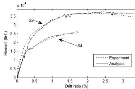
Fig.7 Comparison of moment-drift ratio relations between experimental and analytical results for unbonded PT slab-column connections
