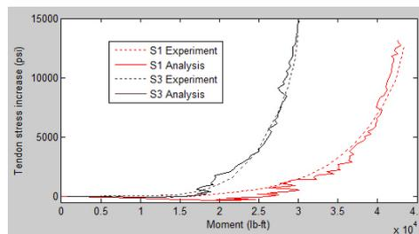
Fig.8 Comparison of moment-tendon stress increase relations from analytical and test results of unbonded PT slab-column connections
