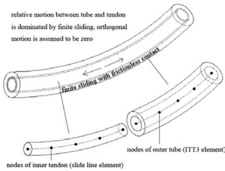
Fig.1 Modeling of unbonded PT tendons using the contact element model
