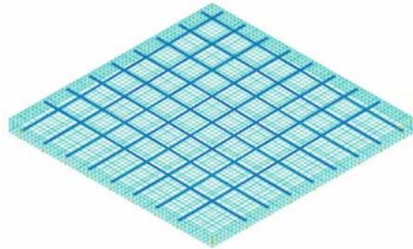
Fig.4 Elements used for unbonded PT slab analysis
