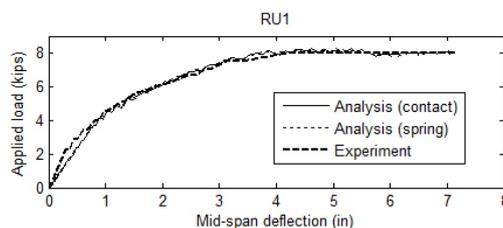
Fig.6 Comparison between the contact formulation and spring system model
