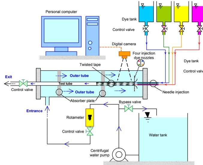
Fig. 2 Schematic diagram of flow visualization setup
