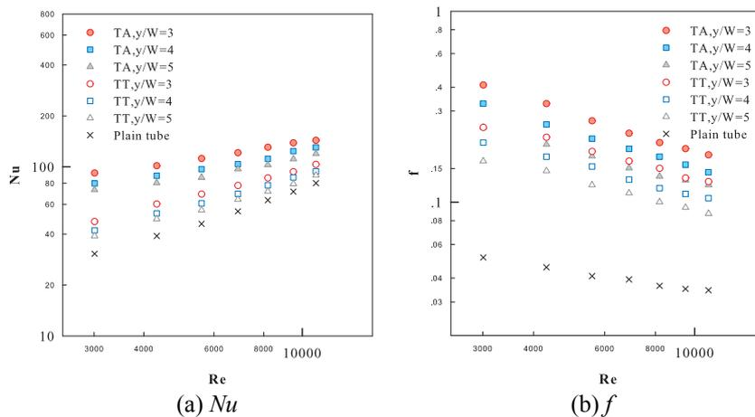
Fig. 5 Variation of Nusselt number and friction factor with Reynolds number
