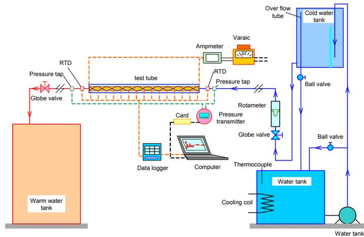
Fig. 3 Schematic diagram of experimental heat transfer setup
