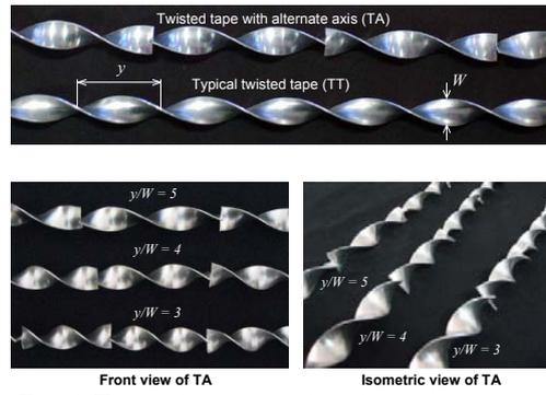
Fig. 1 Twisted tapes used in the present work
