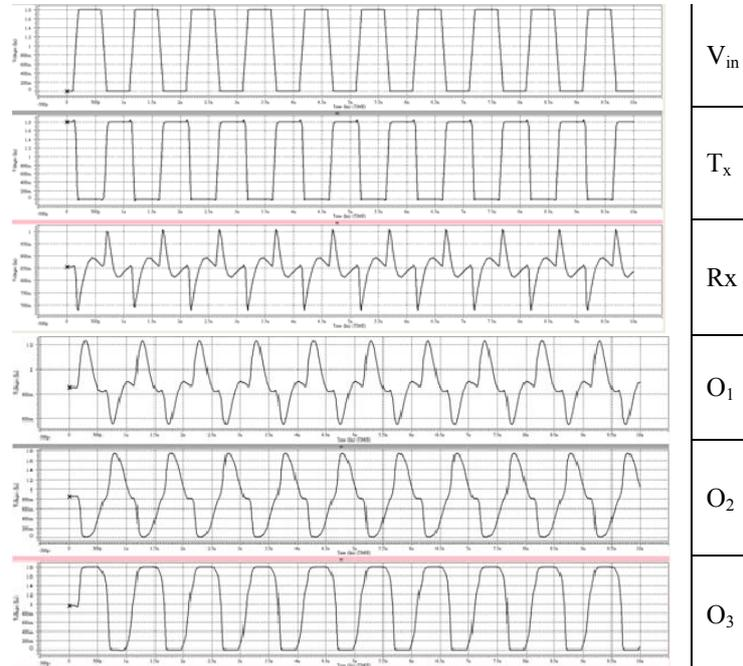
Fig. 8 HSPICE simulation results for capacitive coupling interconnection.
