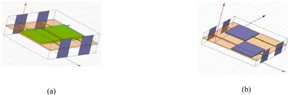
Figure 2. Structure representing coupling channels in top-faced CMOS stacks for (a) parallel type and (b) butterfly difference type.
