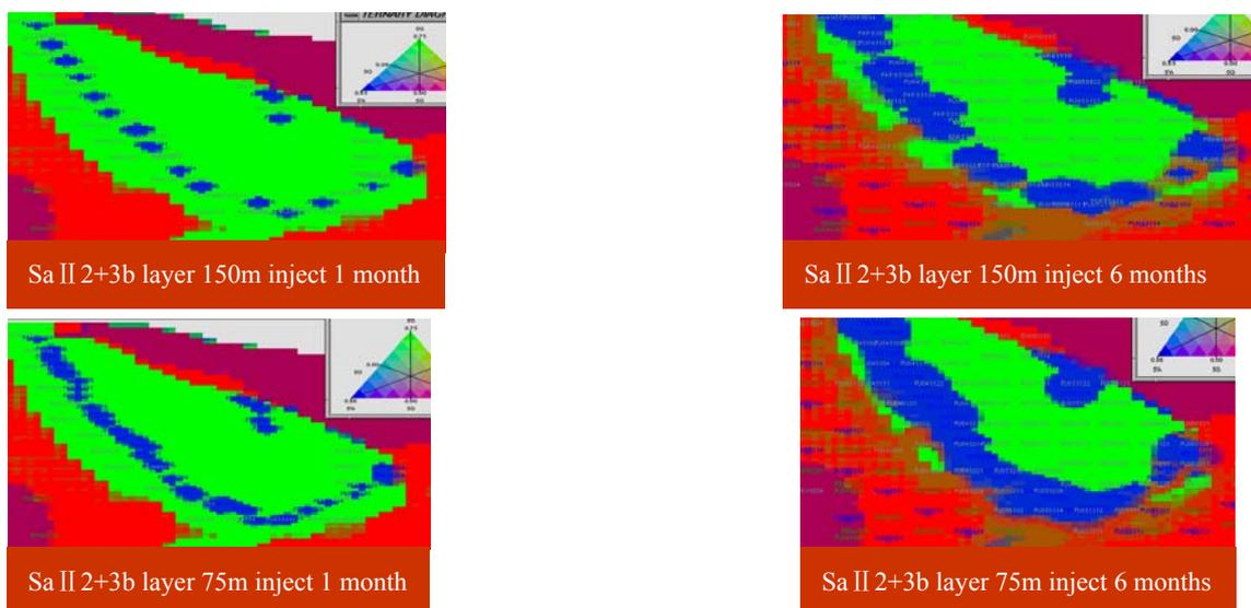
Figure 2 Comparison chat of 150m and 75m well space forming polymer barrier wall
