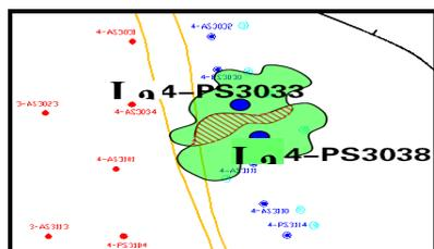
Figure 3 well La4-PS3033, La4-PS3038 displacement frontal
