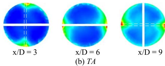
Fig. 3 Contour plot of fluid temperature at  $Re \approx 500$
