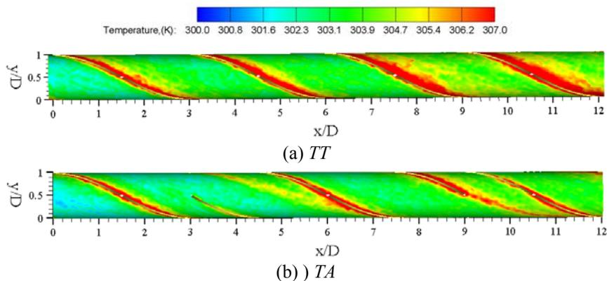
Fig. 4 Wall temperature around inner tube with twisted tape at  $Re \approx 500$
