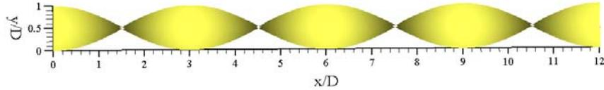
Fig. 1 Twisted tape geometry
