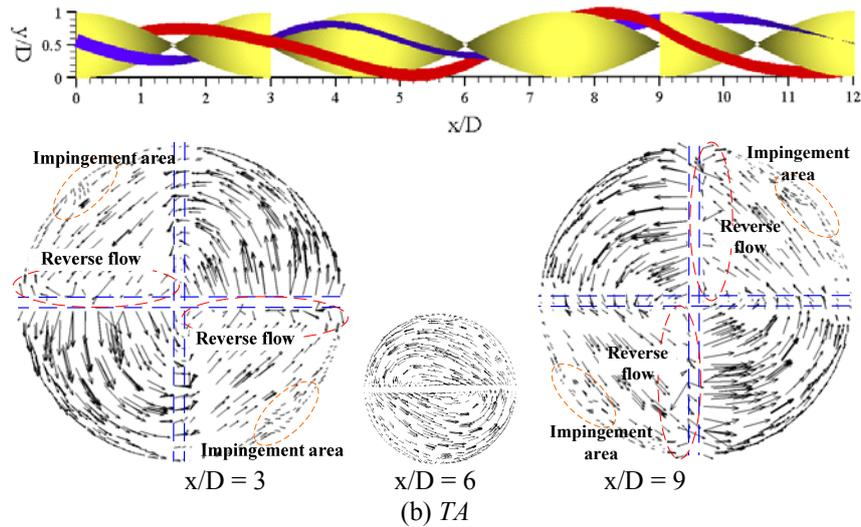
Fig. 2 Pathline and velocity vector in a tube with twisted tape
