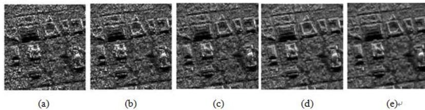
Fig 4. SAR image Denoising (a) noisy image of variance 0.05 (b) DBA filter output (c) Lee filter output (d) Sigma filter output (e) Proposed filter Output
