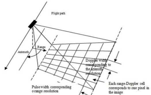
Fig 1. Principle of SAR Processing
