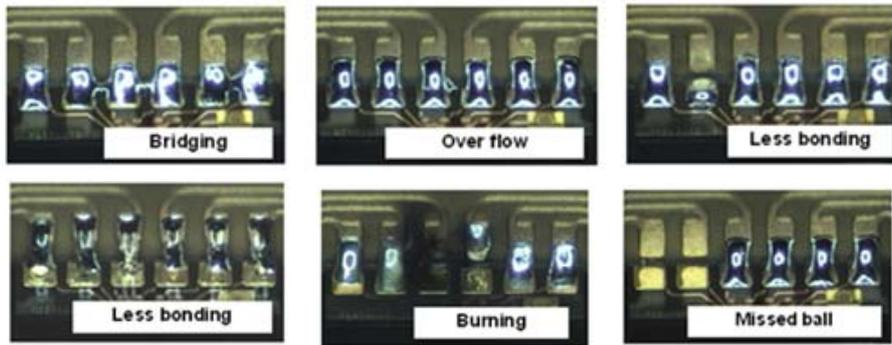
Fig. 1: The solder jet bonding defect type
