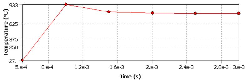
Fig. 5: The Maximum temperature profiles for 2 laser pulse
