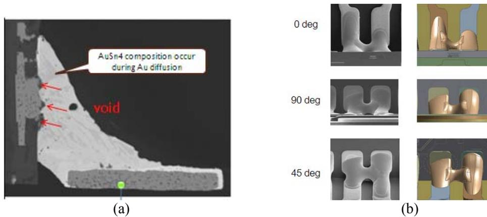
Fig. 4: a: The void happen in SAC305 on gold plating surface, b: The bridging model validation
