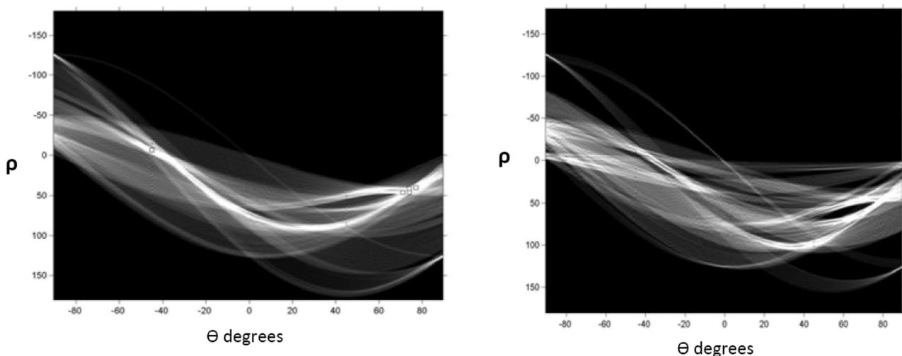
Fig.6 (a, b): Line detection on real images using the Hough transformation.
