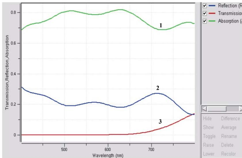
Fig. 5: Reflectance, Transmittance and Absorption of InP/InGaAs/InGaSb at 45° incidence [7].
