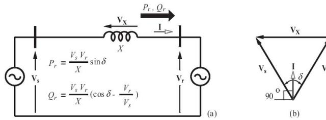
Fig 1. (a) Power transmission system (b) Phasor diagram
