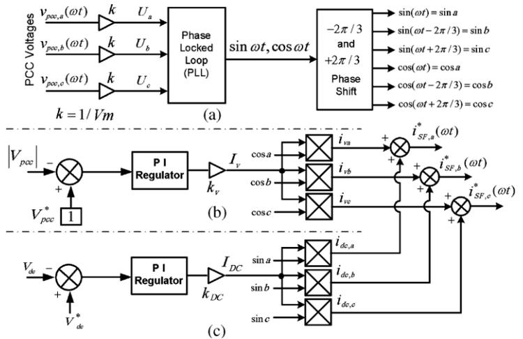
Fig .6: SF as STATCOM—controller diagrams.
