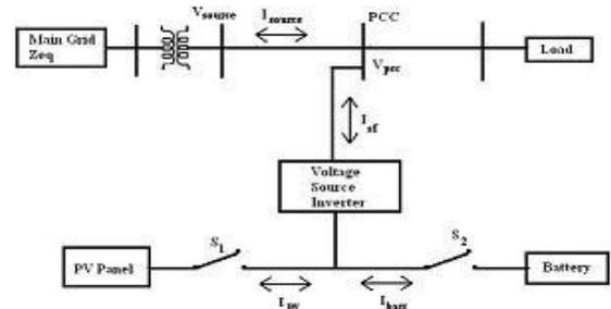
Fig.2 Solar farm inverter as the battery charger system
