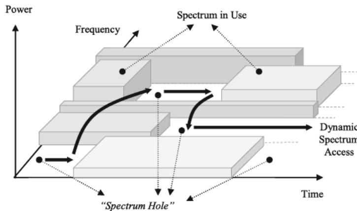
Fig. 1: Spectrum Hole Concept
