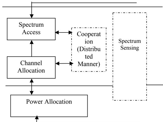
Fig. 3: Functional Block diagram for Spectrum sharing – Wireless Networks
