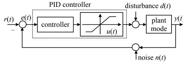
Fig. 1: A typical PID control
