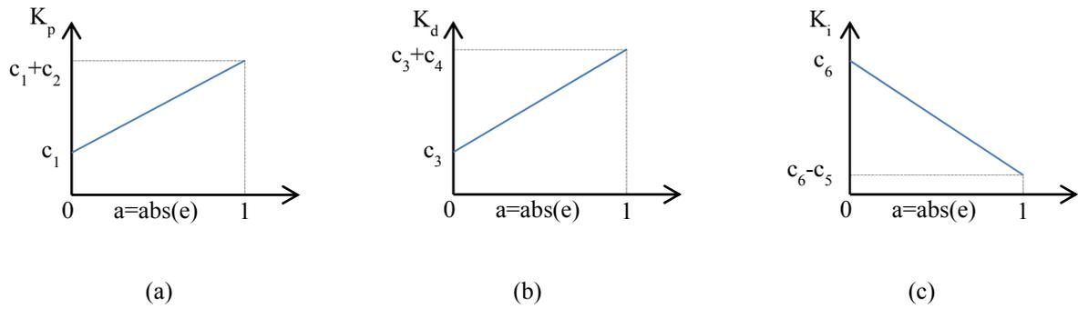
Fig. 3: Change of  $K_p$ ,  $K_d$  and  $K_i$  to absolute of error
