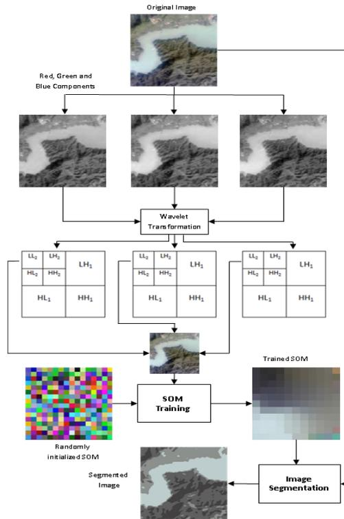
Figure 1: Flow diagram of segmentation process using SOM and wavelets
