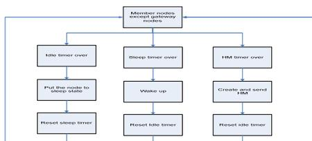
Figure 2: State diagram for nodes with concern to energy
