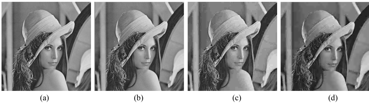
Fig. 3: (a) (b) The Lena image with 0.915 bpp before/after deblocking (c) (d) The Lena image with 0.279 bpp before/after deblocking
