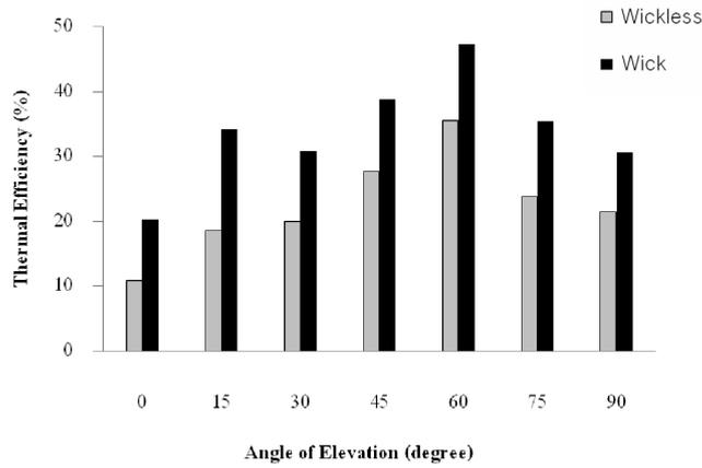
Figure 5. Variation of heat pipe thermal efficiency with tilt angle of heat pipe at water flow rate of 1.0 l/min
