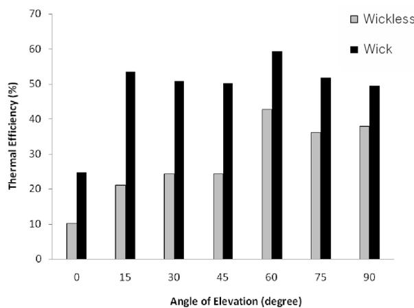
Figure 4. Variation of heat pipe thermal efficiency with tilt angle of heat pipe at water flow rate of 0.5 l/min
