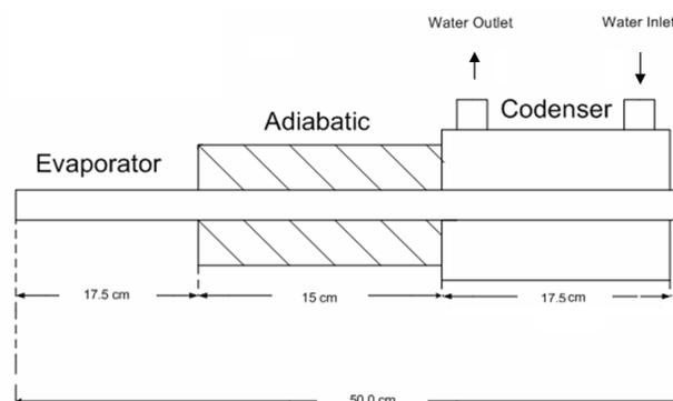
Figure 2. The heat pipe dimensions
