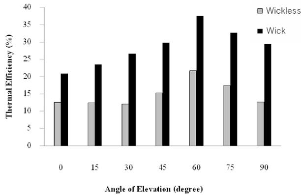
Figure 6. Variation of heat pipe thermal efficiency with tilt angle of heat pipe at water flow rate of 1.5 l/min
