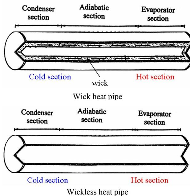
Figure 1. Wicked and wickless heat pipes
