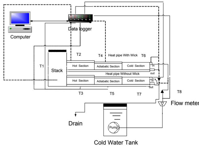
Figure 3. Schematic diagram of the testing facility
