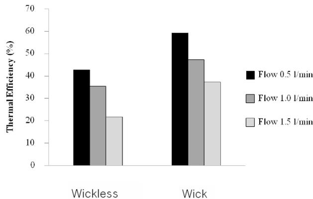
Figure 7. Variation of heat pipe thermal efficiency with heat pipe configuration (wick and wickless) for different flow rate
