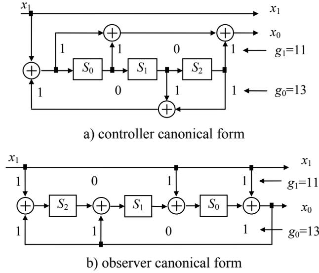
Fig.1 The scheme of the component code of the TC specified in the standard 3GPP-RAN, having the generator matrix  $G_{3gpp}=[11 \ 13]$ .
