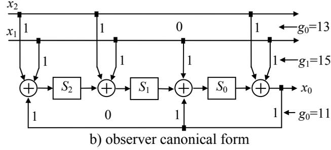
Fig.2 The scheme of the component code of the TC specified in the standard DVB-RCS, having the generator matrix  $G_{DVB}=[13\ 15\ 11]$ .
