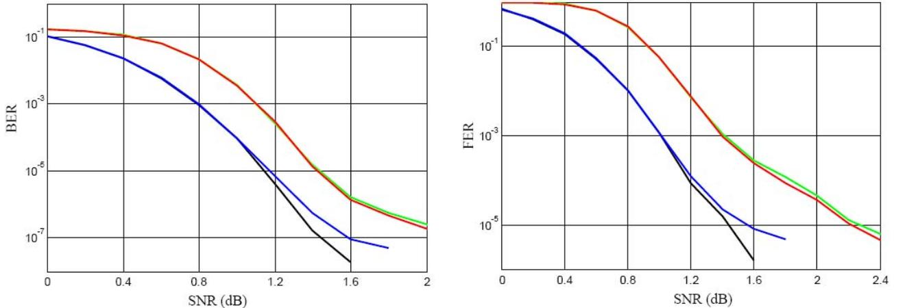
Fig. 5 BER/FER versus SNR performances for the TCs:  $\mathcal{TC}_{3gppd}$  (black),  $\mathcal{TC}_{3gppd}$  (blue),  $\mathcal{TC}_{DVB}$  (green) and  $\mathcal{TC}_{DVBd}$  (red) in the tail biting case.
