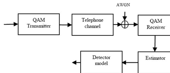
Figure 1. Model of data transmission
