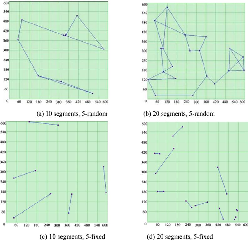
Figure 6. The deployment of backup fibers for different instances of the MPMDC problem
