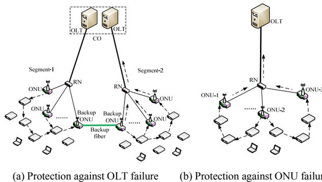
Figure 2. Illustration of the protection scheme
