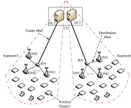
Figure 1. The WOBAN architecture with two segments
