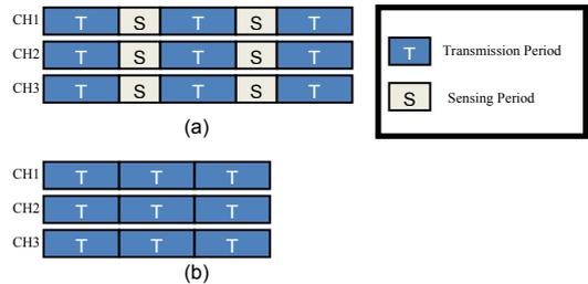
Figure 3. (a) Sensing cycle for existing CR networks (b) Sensing cycle for proposed stand-alone architecture for smart buildings.
