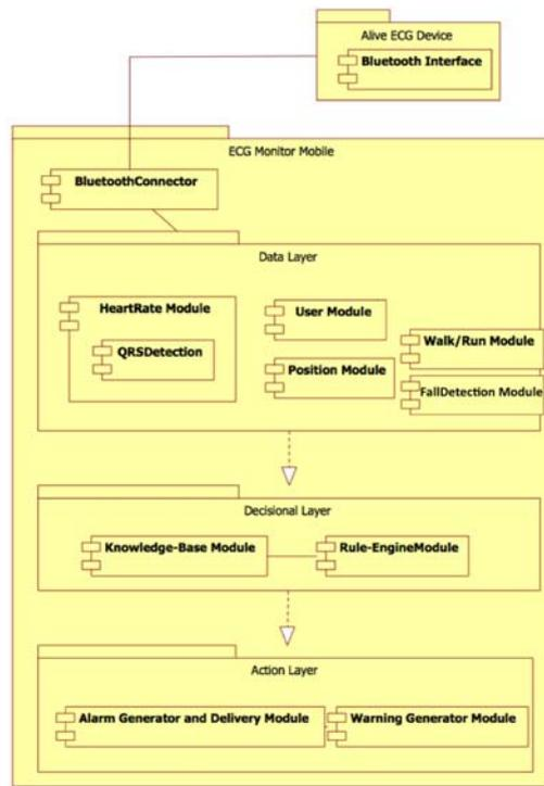
Figure 1. Component diagram of the proposed advanced mobile system
