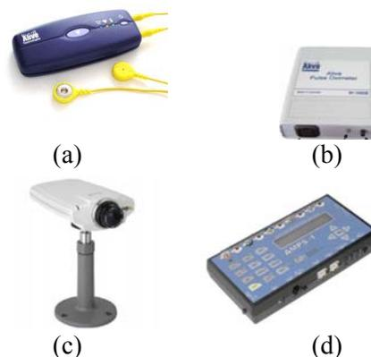
Figure 2. Hardware devices used to test system performances : (a) Alive Heart Monitor; (b) Alive Oximeter Monitor; (c) Axis 210A IP Network Camera; (d) Datrend AMPS-1 Patient Simulator
