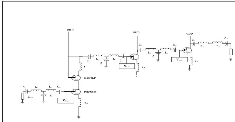
Fig. 3: Schematic diagram of proposed LNA
