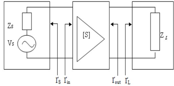
Fig. 2: I/O circuit of 2-port network
