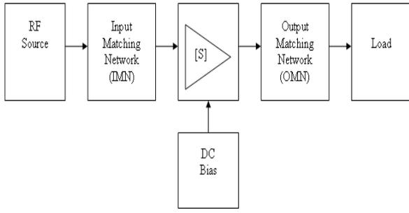
Fig. 1: Typical amplifier designed
