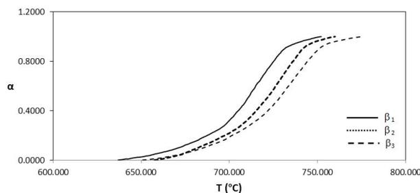
Fig. 2: Reaction progress curve in 3 reaction rate ( $\beta_1=7$ ,  $\beta_2=10$ ,  $\beta_3=15$  degree on minute).
