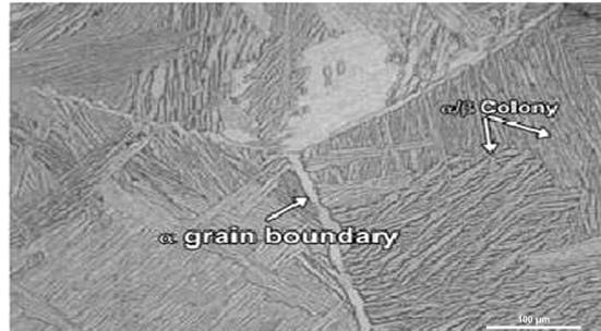
Fig. 2: Microstructure of casted sample.
